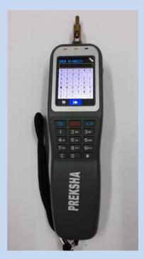
Breath Analyzer Model: ALERT PLUS-15 { With Spl. Attachment for Blow by Normal STRAW }
